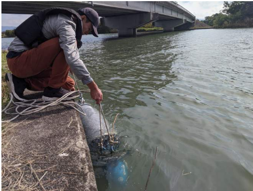
Figure 22 Collecting solids with the device (Albatross Mark VI)
