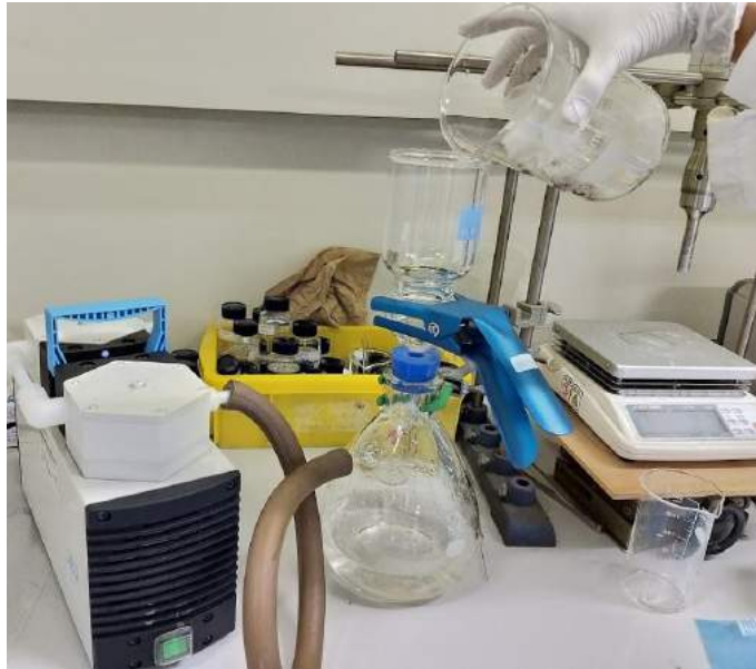
Figure 23 Extracting by hydrochloric acid treatment and filtration
