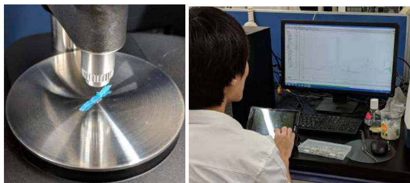
Figures 11,12 Analysis of components using FT-IR
